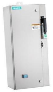
Non-reversing motor starter Size 0 Three phase full voltage Solidstate overload relay OLRelay amp range 5.5-22A 190-220/220-240V 50/60HZ coil Combination type 25Amp circuit breaker Encl NEMA type 4X 316 S-steel Water/dust tight noncorrosive Standard width enclosure
