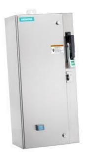
Non-reversing motor starter Size 0 Three phase full voltage Solidstate overload relay OLRelay amp range 5.5-22A 380-440/440-480V 50/60HZ coil Combination type 25Amp circuit breaker Encl NEMA type 4X 316 S-steel Water/dust tight noncorrosive Standard width enclosure
