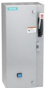
Non-reversing motor starter Size 1 Three phase full voltage Solidstate overload relay OLRelay amp range 0.75-3.4A 24Vdc coil Combination type 3Amp circuit breaker Enclosure NEMA type 1 Indoor general purpose use Standard width enclosure
