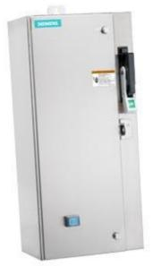
Non-reversing motor starter Size 1 3/4 Three phase full voltage Amb compensate bimetal OLrelay Contactor amp rating 40Amp 208VAC 60HZ coil Combination type 40AMP circuit breaker Encl NEMA type 4X 304 S-steel Water/dust tight noncorrosive Standard width enclosure
