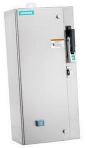
Non-reversing motor starter Size 1 3/4 Three phase full voltage Amb compensate bimetal OLrelay Contactor amp rating 40Amp 550/575-600 50/60HZ coil Combination type 40AMP circuit breaker Encl NEMA type 4X 304 S-steel Water/dust tight noncorrosive Standard width enclosure
