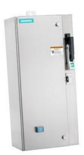
Non-reversing motor starter Size 1 3/4 Three phase full voltage Amb compensate bimetal OLrelay Contactor amp rating 40Amp 110V 50HZ / 120V 60HZ coil Combination type 40AMP circuit breaker Encl NEMA type 4X 304 S-steel Water/dust tight noncorrosive Standard width enclosure
