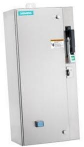
Non-reversing motor starter Size 1 3/4 Three phase full voltage Amb compensate bimetal OLrelay Contactor amp rating 40Amp 240V 50HZ / 277V 60HZ coil Combination type 40AMP circuit breaker Encl NEMA type 4X 304 S-steel Water/dust tight noncorrosive Standard width enclosure
