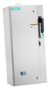
Non-reversing motor starter Size 1 3/4 Three phase full voltage Amb compensate bimetal OLrelay Contactor amp rating 40Amp 110-120/220-240VAC 60HZ coil Combination type 50Amp circuit breaker Encl NEMA type 4X 304 S-steel Water/dust tight noncorrosive Standard width enclosure
