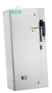
Non-reversing motor starter Size 1 3/4 Three phase full voltage Amb compensate bimetal OLrelay Contactor amp rating 40Amp 208VAC 60HZ coil Combination type 50Amp circuit breaker Encl NEMA type 4X 304 S-steel Water/dust tight noncorrosive Standard width enclosure
