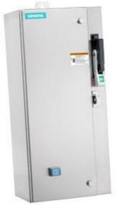
Non-reversing motor starter Size 1 3/4 Three phase full voltage Amb compensate bimetal OLrelay Contactor amp rating 40Amp 550/575-600 50/60HZ coil Combination type 50Amp circuit breaker Encl NEMA type 4X 304 S-steel Water/dust tight noncorrosive Standard width enclosure
