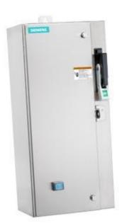
Non-reversing motor starter Size 1 3/4 Three phase full voltage Amb compensate bimetal OLrelay Contactor amp rating 40Amp 110V 50HZ / 120V 60HZ coil Combination type 50Amp circuit breaker Encl NEMA type 4X 304 S-steel Water/dust tight noncorrosive Standard width enclosure
