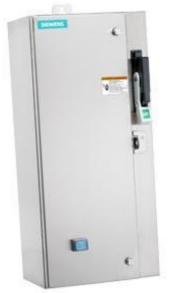
Non-reversing motor starter Size 1 3/4 Three phase full voltage Amb compensate bimetal OLrelay Contactor amp rating 40Amp 240V 50HZ / 277V 60HZ coil Combination type 50Amp circuit breaker Encl NEMA type 4X 304 S-steel Water/dust tight noncorrosive Standard width enclosure
