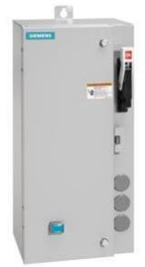
Non-reversing motor starter Size 2 Three phase full voltage Amb compensate bimetal OLrelay Contactor amp rating 45Amp 110V 50HZ / 120V 60HZ coil Combination type 50Amp circuit breaker Enclosure NEMA type 4/12 Water/dust tight for outdoors Standard width enclosure
