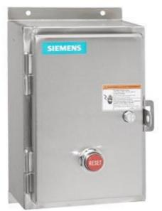
Reversing motor starter Size 2 Three phase full voltage Amb compensate bimetal OLrelay Contactor amp rating 45Amp 208VAC 60HZ coil Non-combination type Encl NEMA type 4X 304 S-steel Water/dust tight non-corrosive
