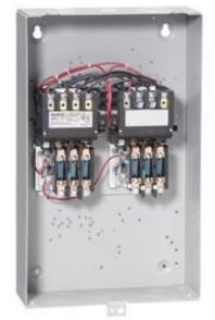
2-speed 3-phase motor starter Size 2 1/2 Two separate windings Constant or variable torque Amb compensate bimetal OLrelay Contactor amp rating 60Amp 110-120/220-240VAC 60HZ coil Noncombination type Enclosure NEMA type (open) No enclosure
