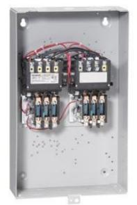
2-speed 3-phase motor starter Size 2 1/2 Two separate windings Constant or variable torque Amb compensate bimetal OLrelay Contactor amp rating 60Amp 110V 50HZ / 120V 60HZ coil Noncombination type Enclosure NEMA type (open) No enclosure
