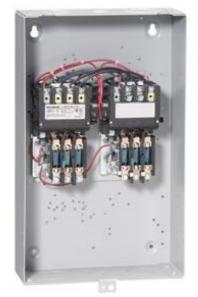
2-speed 3-phase motor starter Size 3 Two separate windings Constant or variable torque Amb compensate bimetal OLrelay Contactor amp rating 90 AMP 110-120/220-240VAC 60HZ coil Noncombination type Enclosure NEMA type (open) No enclosure
