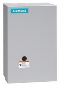
2-speed 3-phase motor starter Size 3 Two separate windings Constant or variable torque Amb compensate bimetal OLrelay Contactor amp rating 90 AMP 110V 50HZ / 120V 60HZ coil Noncombination type Enclosure NEMA type 1 Indoor general purpose use
