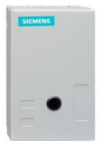
Non-reversing NEMA contactor, Size 00, Three phase full voltage, Contactor amp rating 9A, 3 wire (NO aux included), 208VAC 60Hz coil, Non-combination type, Enclosure NEMA type 1, Indoor general purpose use, Standard width enclosure
