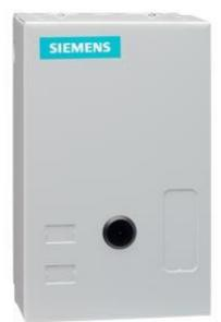
Non-reversing NEMA contactor, Size 0, 4 power poles, Contactor amp rating 18A, 3 wire (NO aux included), 380-440/440-480V 50/60Hz coil, Non-combination type, Enclosure NEMA type 1, Indoor general purpose use, Standard width enclosure
