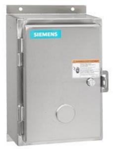
Non-reversing NEMA contactor, Size 0, 4 power poles, Contactor amp rating 18A, 3 wire (NO aux included), 110-120/220-240VAC 60Hz coil, Non-combination type, Encl NEMA type 4X 304 S-Steel, Water/dust tight noncorrosive, Standard width enclosure
