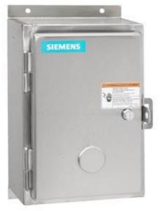
Non-reversing NEMA contactor, Size 0, 4 power poles, Contactor amp rating 18A, 3 wire (NO aux included), 190-220/220-240V 50/60Hz coil, Non-combination type, Encl NEMA type 4X 304 S-Steel, Water/dust tight noncorrosive, Standard width enclosure
