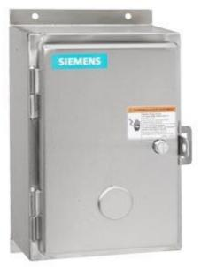
Non-reversing NEMA contactor, Size 0, Three phase full voltage, Contactor amp rating 18A, 3 wire (NO aux included), 208VAC 60Hz coil, Non-combination type, Encl NEMA type 4X 304 S-Steel, Water/dust tight noncorrosive, Standard width enclosure
