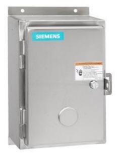
Non-reversing NEMA contactor, Size 0, Three phase full voltage, Contactor amp rating 18A, 3 wire (NO aux included), 380-440/440-480V 50/60Hz coil, Non-combination type, Encl NEMA type 4X 304 S-Steel, Water/dust tight noncorrosive, Standard width enclosure
