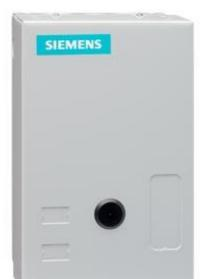
Non-reversing NEMA contactor, Size 1, Single phase full voltage, Contactor amp rating 27A, 3 wire (NO aux included), 110V 50Hz / 120V 60Hz coil, Non-combination type, Enclosure NEMA type 1, Indoor general purpose use, Standard width enclosure
