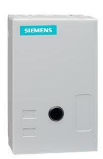
Non-reversing NEMA contactor, Size 1, 4 power poles, Contactor amp rating 27A, 3 wire (NO aux included), 208VAC 60Hz coil, Noncombination type, Enclosure NEMA type 1, Indoor general purpose use, Standard width enclosure
