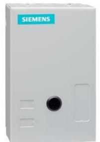
Non-reversing NEMA contactor, Size 1, 4 power poles, Contactor amp rating 27A, 3 wire (NO aux included), 24VAC 50-60Hz coil, Noncombination type, Enclosure NEMA type 1, Indoor general purpose use, Standard width enclosure
