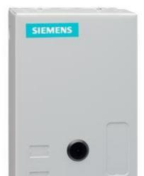
Non-reversing NEMA contactor, Size 1, Three phase full voltage, Contactor amp rating 27A, 3 wire (NO aux included), 24VAC 50-60Hz coil, Non-combination type, Enclosure NEMA type 1, Indoor general purpose use, Standard width enclosure
