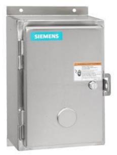
Non-reversing NEMA contactor, Size 1, Three phase full voltage, Contactor amp rating 27A, 3 wire (NO aux included), 220-240/440-480VAC 60Hz coil, Non-combination type, Encl NEMA type 4X 304 S-Steel, Water/dust tight noncorrosive, Standard width enclosure
