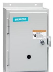
Non-reversing NEMA contactor, Size 1, Three phase full voltage, Contactor amp rating 27A, 3 wire (NO aux included), 208VAC 60Hz coil, Non-combination type, Enclosure NEMA type 12, Dust/drip proof for indoors, Extra-wide enclosure
