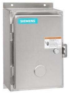
Non-reversing contactor, Size 1 3/4, 4 power poles, Contactor amp rating 40A, 3 wire (NO aux included), 380-440/440-480V 50/60Hz coil, Non-combination type, Encl NEMA type 4X 304 S-Steel, Water/dust tight noncorrosive, Standard width enclosure
