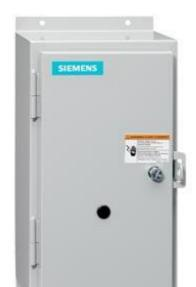
Non-reversing contactor, Size 2 1/2, Single phase full voltage, Contactor amp rating 60A, 3 wire (NO aux included), 190-220/220-240V 50/60Hz coil, Non-combination type, Enclosure NEMA type 12, Dust/drip proof for indoors, Standard width enclosure
