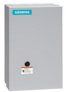
Reversing NEMA contactor Size 0 Three phase full voltage Contactor amp rating 18Amp 3 w 110V 50HZ / 120V 60HZ coil Non-combination type Enclosure NEMA type 1 Indoor general purpose use Standard width enclosure
