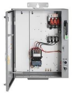
Pump control panel, Size 2 1/2, Three phase full voltage, Solid-state overload relay, OLR amp range 25-100A, 24VAC 50-60Hz coil, Standard type contactor, 100A fusible disconnect, 100A/600V fuse clip, HOA Sel Sw. & Start P.B., Enclosure NEMA type 3/3R, Weather proof outdoor use
