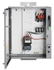
Pump control panel, Size 2 1/2, Three phase full voltage, Solid-state overload relay, OLR amp range 25-100A, 208VAC 60Hz coil, Standard type contactor, 60A fusible disconnect, 60A/600V fuse clip, HOA Sel Sw. & Start P.B., Enclosure NEMA type 3/3R, Weather proof outdoor use
