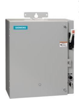
Pump control panel, Size 2 1/2, Three phase full voltage, Solid-state overload relay, OLR amp range 25-100A, 190-220/220-240V 50/60Hz coil, Standard type contactor, 60A fusible disconnect, 60A/600V fuse clip, HOA Sel Sw. & Start P.B., Enclosure NEMA type 3/3R, Weather proof outdoor use
