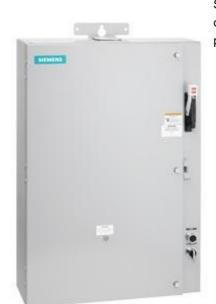
Pump control panel, Size 3, Three phase full voltage, Solid-state overload relay, OLR amp range 25-100A, 24VAC 50-60Hz coil, Standard type contactor, 200A fusible disconnect, 200A/600V fuse clip, HOA Sel Sw. & Start P.B., Enclosure NEMA type 3/3R, Weather proof outdoor use
