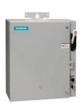
Pump control panel, Size 3, Three phase full voltage, Solid-state overload relay, OLR amp range 25-100A, 190-220/220-240V 50/60Hz coil, Standard type contactor, 100A fusible disconnect, 100A/600V fuse clip, HOA Sel Sw. & Start P.B., Enclosure NEMA type 3/3R, Weather proof outdoor use
