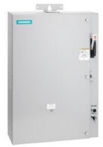
Pump control panel, Size 3, Three phase full voltage, Solid-state overload relay, OLR amp range 25-100A, 240V 50Hz / 277V 60Hz coil, Standard type contactor, 100A fusible disconnect, 100A/600V fuse clip, HOA Sel Sw. & Start P.B., Enclosure NEMA type 3/3R, Weather proof outdoor use
