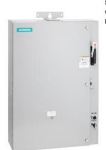
Pump control panel, Size 3, Three phase full voltage, Solid-state overload relay, OLR amp range 25-100A, 24VAC 50-60Hz coil, Standard type contactor, 100A fusible disconnect, 100A/250V fuse clip, HOA Sel Sw. & Start P.B., Enclosure NEMA type 3/3R, Weather proof outdoor use
