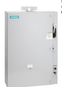
Pump control panel, Size 3 1/2, Three phase full voltage, Solid-state overload relay, OLR amp range 50-200A, 208VAC 60Hz coil, Standard type contactor, 200A fusible disconnect, 200A/600V fuse clip, HOA Sel Sw. & Start P.B., Enclosure NEMA type 3/3R, Weather proof outdoor use
