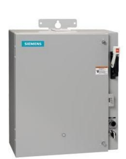
Pump control panel, Size 3 1/2, Three phase full voltage, Solid-state overload relay, OLR amp range 50-200A, 190-220/220-240V 50/60Hz coil, Standard type contactor, 200A fusible disconnect, 200A/600V fuse clip, HOA Sel Sw. & Start P.B., Enclosure NEMA type 3/3R, Weather proof outdoor use
