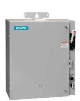
Pump control panel, Size 4, Three phase full voltage, Solid-state overload relay, OLR amp range 50-200A, 190-220/220-240V 50/60Hz coil, Standard type contactor, 200A fusible disconnect, 200A/600V fuse clip, HOA Sel Sw. & Start P.B., Enclosure NEMA type 3/3R, Weather proof outdoor use
