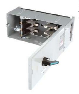
Siemens Low Voltage Circuit Protection Panelboard/Switchboard Units. Type: VB PANELBOARD UNITS Std: UL V. Rating: 600V A. Rating: 100A Number of poles: 2P F. Rating: 60Hz Action: SINGLE THROW Mounting: INSIDE PANEL BOARD. O. Cycles: 10000 O. Temperature: (-20F-120F) AMBIENT TEMPERATURE
