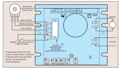
PWM SAFETY WARNING! This control does not contain protection circuitry to prevent full speed runaway in the event of main power transistor failure. However, an optional Product Safety Module (PSM) (P/N 9995) can be installed to prevent full speed runaway. If a PSM is not used, the installer of this product should take proper precautions to include other means, such as mechanical disconnects, warning notices, etc., to protect the operator of the machine involved.
