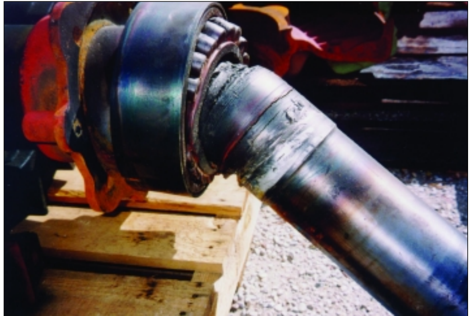
Motor failed due to mismatched and over-tightened sheaves causing excessive heat and melting motor shaft.
