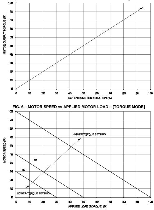
FIG. 5 - MOTOR OUTPUT TORQUE vs POTENTIOMETER ROTATION - [TORQUE MODE]
