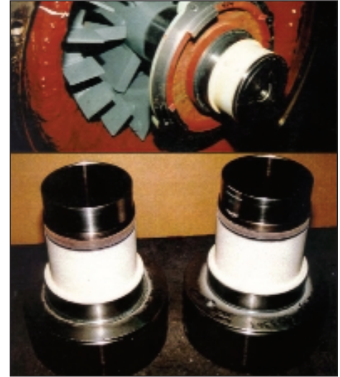
Ceramic or aluminum oxide spray is one method of insulating. Above, an opposite drive end bearing journal, and below, vertical motor bearing carriers, all of which have been insulated with ceramic spray.
