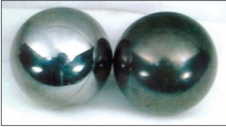
When rotational speed varies, the shaft currents may cause a dull, frosted appearance instead of fluting.
